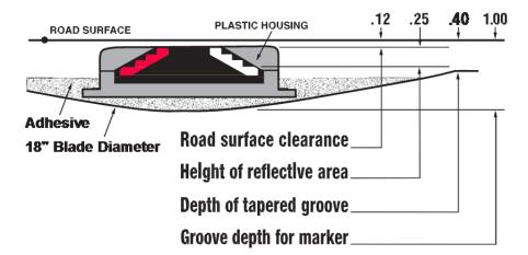
**D. Location and Spacing.** Install the markers in the pattern for high reflectivity with two (2) IPMs per groove. Locate and space markers as shown in the current standard drawings or sepias (note: use Inlaid Pavement Markers wherever Type V Pavement Markers are called for). Do not install markers on bridge decks. Do not install a marker
